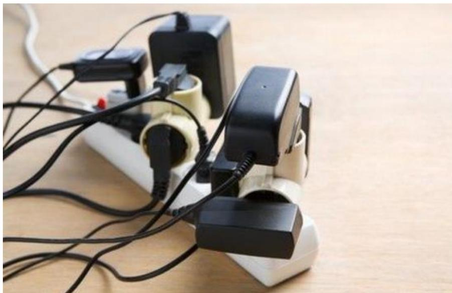
**Do you have a damaged electricity cord?** If you are using an appliance which has a visibly damaged cord, this may be causing the problem. A damaged cord can create an improper connection and can cause the RCD to trip your circuits.
